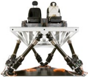
6 DOF ride and comfort test system
