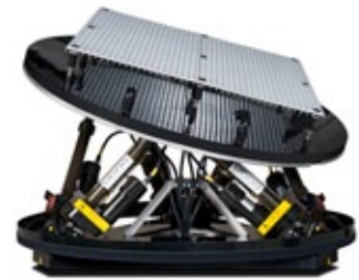
6 DOF antenna test system
