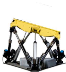
6 DOF fuel tank test system
