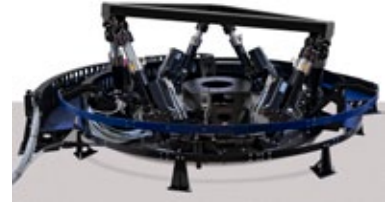
7 DOF motion base with yaw table to simulate city driving
