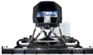
7 DOF driving simulator with lateral rail for vehicle dynamics research or advanced driver assistance
