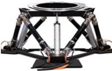
6 DOF tank turret test system with pneumatic assist, capable of handling payloads up to 23 tons
